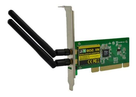
WiFi cards can be **external** or **internal**. If a WiFi card is not installed in your computer, then you may purchase a USB antenna attachment and have it externally connect to your USB port, or have an antenna-equipped expansion card installed directly to the computer (as shown in the figure given above). For laptops, this card will be a PCMCIA card which you insert to the PCMCIA slot on the laptop.
